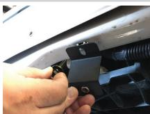
Measure rivet nut hole locations on the Z-hanger brackets. The center-to-center distance should be approximately 7 7/16". Adjust as needed.
