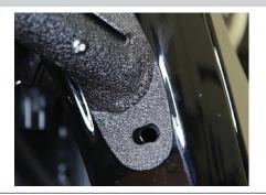
Remove the flare and drill 25/64" OR 10mm holes as needed, to fit the M6 threaded metal inserts supplied with the ARIES fender flares.
