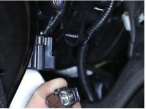
Remove the plastic fender flare support by removing the hex head bolts holding it in place.
