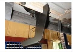
Repeat steps 2 and 3 to install the middle and rear mounting brackets.
