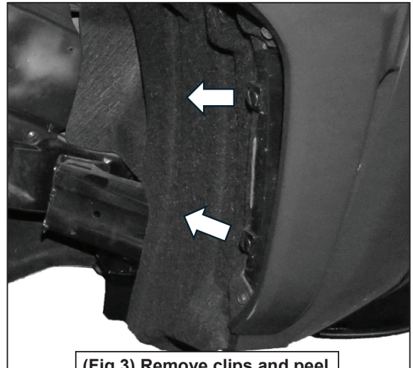
(Fig 3) Remove clips and peel wheel well liner from vehicle
