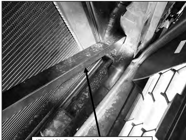
(Fig 13) Driver side top Bracket mounting location behind grille
