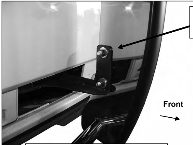
(Fig 11) Driver side Grille Guard installation pictured without plastic panel for instruction purposes only
