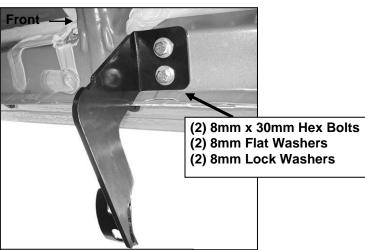
(Fig 3) Driver side center mounting location pictured
