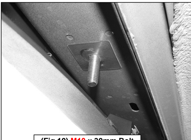
(Fig 10) M10 x 30mm Bolt Plate with Plastic Retainer
