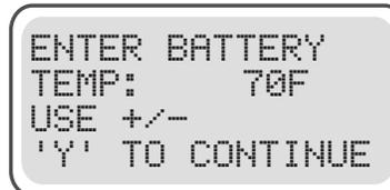
Use the (+Up) and (-Down) Keys to adjust the battery temperature. Press 'Y' to enter.
