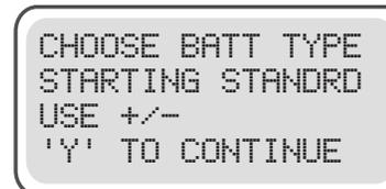
Press the (+Up) or (-Down) key to cycle through the battery types. Press 'Y' when it matches the type of battery you are testing. BATTERY TYPE OPTIONS: STARTING STANDRD STARTING AGM DEEP CYCLE AGM DEEP CYCLE STD
