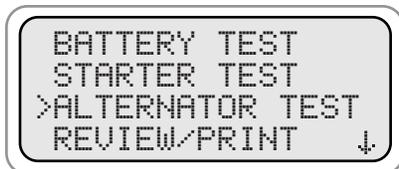
Use the (+Up) and (-Down) arrows to move cursor to the desired test.
