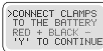
Press 'Y' to continue once the clamps are connected the test will proceed.
