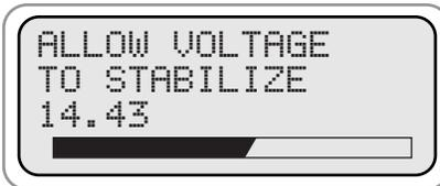
The BVA-300 will allow the voltage to stabilize before starting the test bar at the bottom of the screen that shows the test progress. Be patient, it can take up to 30 seconds for the voltage to stabilize.
