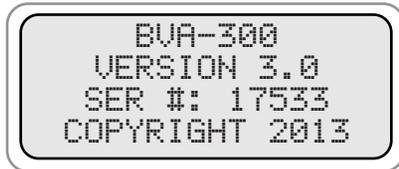
The about screen shows the model number. Firmware revision and the tester serial number. Press any key to go back to the menu.
