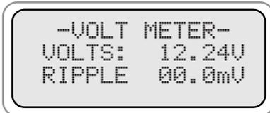
**Note:** If the car is running and the clamps are attached to the battery a high ripple (over 50mV) indicates bad diodes in the alternator.
