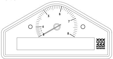
The Display Module is connected to a variety of sensors by a wiring harness. The wiring harness has a 19-way military connector for connection to the Display Module.
