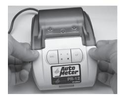
2. Drop in thermal paper roll (as shown). Pull paper out 3" past the cover lid and hold.
