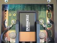
**Illustration 10** Required Gap. Terminal can not touch copper buss bar.
