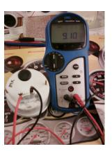
If you get a measurement of 2.9K, you may then send the speedometer into us for service to have an internal circuit modification performed. This modification in most cases will remedy the problem. If you get a measurement of 4.6K or higher, then no modification is needed.
