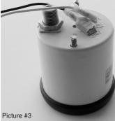
For Mechinical LED lit gauges, you may bend the light terminals down as shown in picture 3. This applies to deep case gauges that measure 1-3/4" from behind the bezel to the end of the case.
