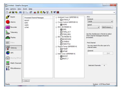
In order to edit or create a CAN message; use the edit protocol tab which will open the CAN template editor. This window can be used to create and edit CAN messages as well as set peak recall settings for CAN channels.
