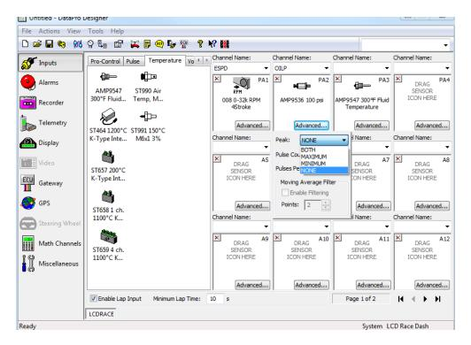
In the advanced tab for other sensors, Peak options can be selected for none, minimum, maximum, or both. These values will show up on the screen when the peak recall switch is pressed.
