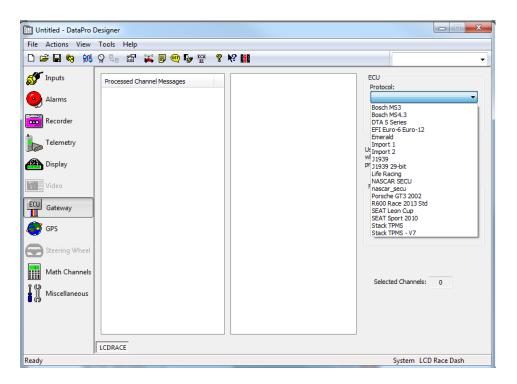
Once the desired protocol is selected, a list of available channels may be enabled for display and recording purposes. When a CAN channel is selected, it will show up in the left hand column and can be seen in the recording, alarms, and display tabs as available channels.
