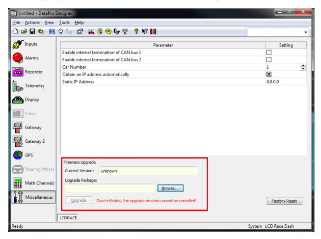
When a connection is made to an LCD dash, the current version number will be reported in the current version field.
