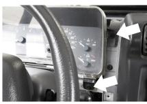
6) (A)Remove the 2 factory wire harness clips by pushing the side tabs in and sliding the clip down. (B) Push the black plastic fastener through the metal, releasing the wire harness.
