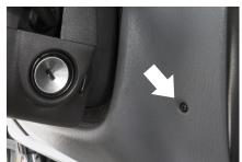
3) Remove the two screws that hold the dash panel below the steering column. There is one screw on each side; one near the headlight switch and one near the ignition switch. Retain the screws, they will be reused during installation.
