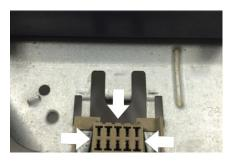
7) Push the side tabs in and slide the clip down to remove the connector from the sheet metal. DO NOT reinstall clips into the dash after you have finished your wiring. The clips will interfere with your new gauges. Secure the clips by using zip ties to keep the wires out of the way.
