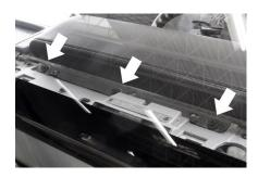
8) After installing your gauges into the panel, mount your new panel. Install the 3 factory screws on top, near the windshield. NOTE: It is important to install these first.
