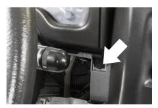
4) Remove the remaining two screws from the bottom of the factory bezel. They are located on the bottom left and bottom right of the factory bezel. Retain the screws, they will be reused in the installation of your new panel.
