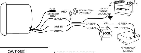
As a safety precaution, the +12V terminal of this product should be fused before connecting it to the 12V ignition switch. We recommend using a 3 Amp, automotive type fuse.
