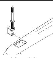
Remove rear stake pocket cover, install rear stake pocket bolt by hooking under bracket inside pocket. Hand tighten the stud thru the hole until the washer (welded to the stud) bottoms out.
