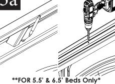
Place the rails onto the truck locating over the stake pocket bolts, the rail can be temporarily hand tightened in place, or held firmly in place while marking. Mark the location of the square hole. Using a hand drill, carefully drill the center of the marked position with a 1/8" drill (pilot hole). Finish drilling rail with a 1/2"
