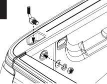
Install rear stake pocket bolt inside pocket. Hand tighten the bolt with lock washer and washer as shown.
