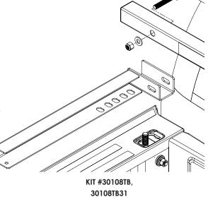
S/8" STEEL NUT, LOCK WASHER AND FLAT WASHER
