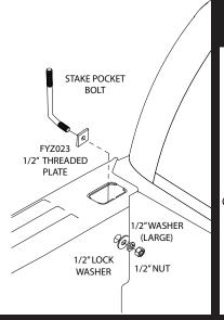
Insert spacer plate over stake pocket bolt as shown, apply adhesive foam opposite to bolt clearance as shown
