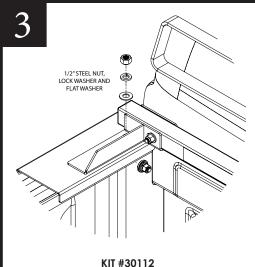
Fasten Backrack Assembly to the Stake pocket bolt as shown.
