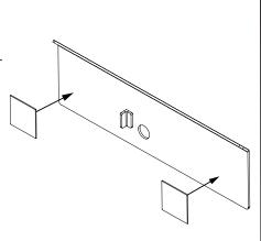
Apply single sided adhesive pads to this side of spacer. Apply BACKRACK decal \*\*Can also be applied as last step to ensure facing outward\*\*
