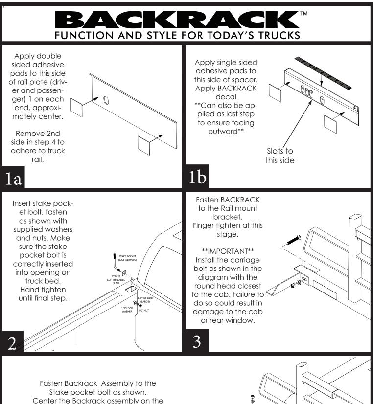
truck and final torque all bolts starting with the nuts on the inside of the truck bed, then the rail mount bracket and finally the main BACKRACK carriage bolt.
