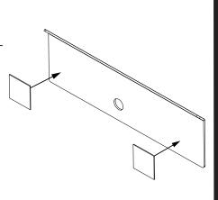
Apply single sided adhesive pads to this side of spacer. Apply BACKRACK decal
