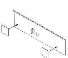
Apply single sided adhesive pads to this side of spacer. Apply BACKRACK decal \*\*Can also be applied as last step to ensure facing outward\*\*
