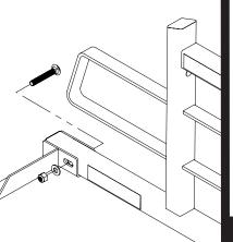
Fasten Backrack Assembly to the Stake pocket bolt as shown. Center the Backrack assembly on the truck and final torque all bolts starting with the nuts on the inside of the truck bed, then the rail mount bracket and finally the main BACKRACK carriage bolt.
