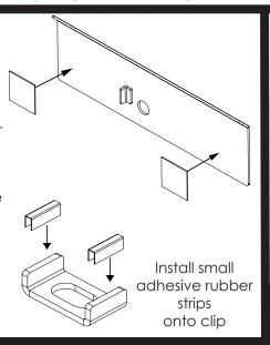
Apply single sided adhesive pads to this side of spacer. Apply BACKRACK decal \*\*Can also be applied as last step to ensure facing outward\*\*
