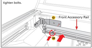
**Removing Front Accessory Rail**: If your Gladiator is equipped with a front accessory rail, it must be removed at this time to allow for the installation of the driver side front mounting bracket (O). Remove the bolts that hold the accessory rail to the bulkhead on both driver and passenger side front corners. If you do not have a front accessory rail, skip to step 4.
