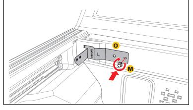
**6** Installing Rear Mounting Brackets: Locate the outlined section on the inside of the bed cap towards the taillight well at the rear of the bed on the driver's side. Cut and remove the outlined section of the bed cap to reveal two threaded holes. Locate the rear mounting bracket (Q) and install two of the M6 flange mounting bolts (M) through the bracket and into the threaded holes.
