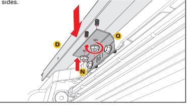
**9 Installing Side Rails**: Apply downward pressure to the driver side rail (B) on to the adaptor rail driver side (D) clamping both together to the truck bed rail. When tightening each clamp (H) make sure the side rail sits flush and seals properly. A second set of hands may help. Repeat on the opposite side using the passenger side rail (C) and the adaptor rail passenger side (E).
