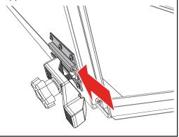
First, prep the buckle ends (I) by peeling off the adhesive liner of the gasket (J).
