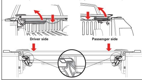
**18** Retighten the cover retainer clamps once the desired fitment is reached. You are ready to drive with your cover in the closed position.
