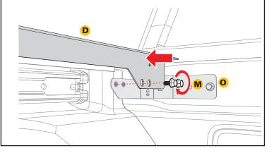
**B** Install the adaptor rail driver side (D) by lining up the studs with the holes in the rear bracket using two M6 flange mounting bolts (M) and two 1/4-20 nuts (N). Repeat on the opposite side using the passenger side adaptor rail (E). Now tighten, using a 7/16" socket in front and rear on both sides.
