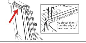
**16** Unfold the cover (A) towards the tailgate. Then confirm each panel is centered side to side and front to back on the truck bed. If adjustments are needed, loosen the cover retainer clamps (G) and shift the cover until positioned correctly. The rear edge of the cover and tailgate seal should rest on top of the tailgate. For proper sealing, the tail panel will overlap by .5".
