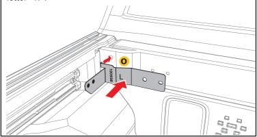
**5** If you **DID** remove the front accessory rail, as mentioned in step 2, proceed to install the accessory rail over the front bracket (O) you just installed aligning the holes in both using one M6 flange mounting bolt (M) through both and into the bulkhead. Repeat on passenger side using the passenger side front mounting bracket (P) labeled with the letter "R". Then
