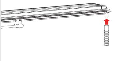
Place the passenger side rail (A) on to the passenger side mounting rail (N) installed in the previous steps. Position the side rail flush with the top edge of the mounting rail. The end of the side rail with the drain tube goes toward the cab of the truck.
