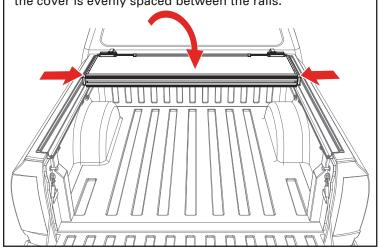
Confirm the retainer clamps (E) are positioned around the side rails (A & B) correctly as shown below. Tighten the retainer clamps by turning them clockwise until the lock washer is secure.
