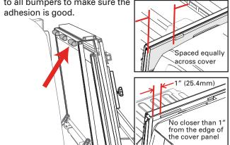
Unfold the cover (C) towards the tailgate. Then confirm each panel is centered side to side and front to back on the truck bed. If adjustments are needed, loosen the cover retainer clamps (E) and shift the cover until positioned correctly. The rear edge of the cover and tailgate seal should rest on top of the tailgate. For proper sealing, the tail panel will overlap by .5".
