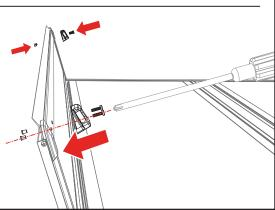
Set the cover (C) in the folded position on the side rails (A & B) towards the cab of the truck. Confirm the cover is evenly spaced between the rails.
