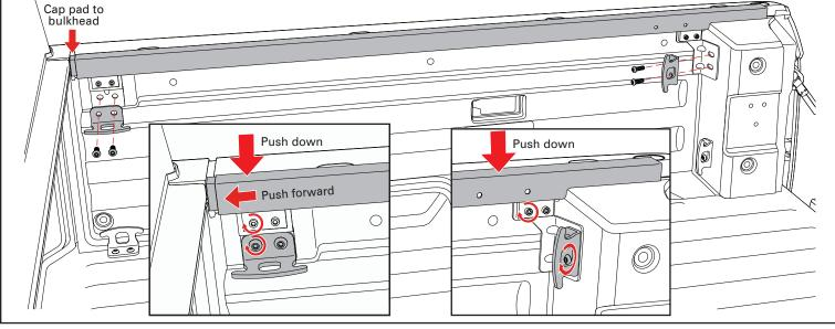
Insert the passenger rail end corner (V) Into the tailgate end of the passenger side mounting rail (N). Do this also on the driver side withVthe driver side mounting rail (M) and the driver rail end corner (U).
