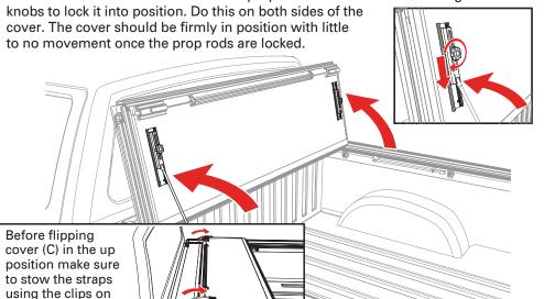
CLOSING COVER: To drive with the cover (C) closed, unhook the buckles and straps from the bulkhead. Stow the straps using the clips on the underside of the folded cover. Fold all panels towards the tailgate making sure that all latches are engaged.
