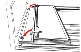
**FLIPPED UP POSITION**: Fold the cover (C) open and lift it until it's vertical or past 90 degrees towards the truck cab. Then release the prop rod that is attached to the rail. Fold the prop rod over and position it firmly against the vertical plate on the underside of the cover. Then slide the prop rod locks downwards and tighten the knobs to lock it into position. Do this on both sides of the
