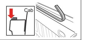
Attach the drain tubes (K) to the front of the side rails (A & B) to allow water to be diverted out of the truck bed via the rail. The opposite end of the drain tubes can be placed behind a bedliner, through the bed plugs, or by drilling a 5/8" hole in the bulkhead.
