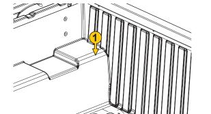
Attach the drain tubes (O) to the front of the side rails (B & C) to allow water to be diverted out of the truck bed via the rail. Drill a 5/8" hole in the top corner of the wheel well as shown in the CAUTION Step (location 1), then run the opposite end of the drain tube through the 5/8" hole.
