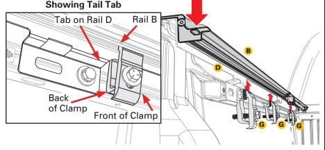
**NOTE:** If the rails are leaning down, have one person stand on the outside of the bed and slightly roll the rails upward while another person slowly snugs the clamps up. If the clamps are tightened too quickly or overtightened, it will cause the rails to lean down.
