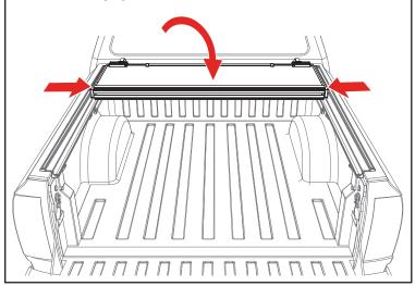
Confirm the retainer clamps (F) are positioned around the side rails (B & C) correctly as shown below. Tighten the retainer clamps by turning them clockwise until the lock washer is secure.
