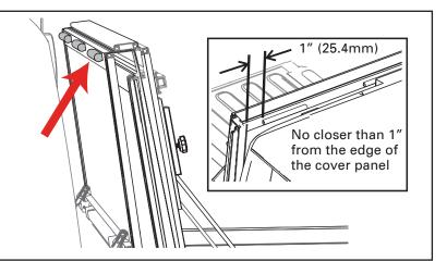
Unfold the cover (A) towards the tailgate. Then confirm each panel is centered side to side and front to back on the truck bed. If adjustments are needed, loosen the cover retainer clamps (F) and shift the cover until positioned correctly. The rear edge of the cover and tailgate seal should rest on top of the tailgate. For proper sealing, the tail panel will overlap by .5".
