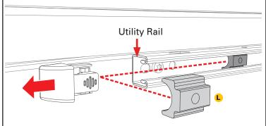
Installing Adaptor Rail: Install adaptor rail driver side (D) with the bolt, washer and lock washer that is attached to the T-nut kit (L) and push the rail all the way toward the cab and the bulkhead. Adjust the t-nuts so they are lined up with the holes in the adaptor rail.
