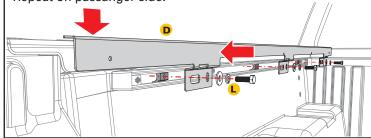
When you get the adaptor rail driver side (D) and T-nut kits (L) lined up you can now tighten the bolts while you are applying downward pressure to the rail. A second set of hands may help. Repeat on the opposite side using the adaptor rail passenger side (E).
