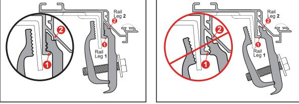
**Water Intrusion**: Make sure the retaining clamps are tight and properly engaged to the side rails. Check that the bulkhead seal is in place and the cover is resting on it. Make sure that all latches are engaged to the side rails and adjust if needed. Check that the side rails are installed flush with the top of the bed rail.
