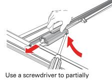
pry open the tab on the latch housing. At the same time slide the housing away from the latch assembly.
