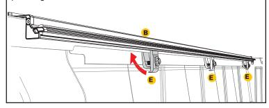
**For Trucks With Cargo Management System**: Remove the factory end caps from both ends of the bulkhead utility rail.
