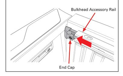
**B** Installing T-nut Kits in Cargo Management System: Remove the factory end cap from tailgate end of the accessory rail. Insert three T-nut kits (J) into the end of the accessory rail and put the end cap back in. Repeat on passenger side.
