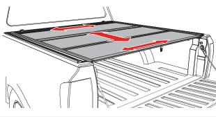
**Power Tailgates:** If your truck has a powered opening or closing tailgate ensure the tailgate functions properly with the cover closed and if needed adjust the cover towards the truck cab.
