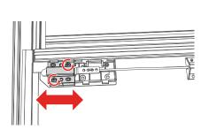
With the latch cover removed, loosen the screws and move the latch bracket to adjust. Retighten the screws. Slide the latch housing back on.
