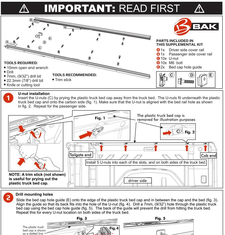
so that the placement of the U-nut underneath can be shown
