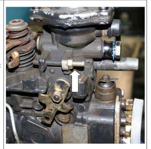
Picture shows cap and extra jam nut removed.
