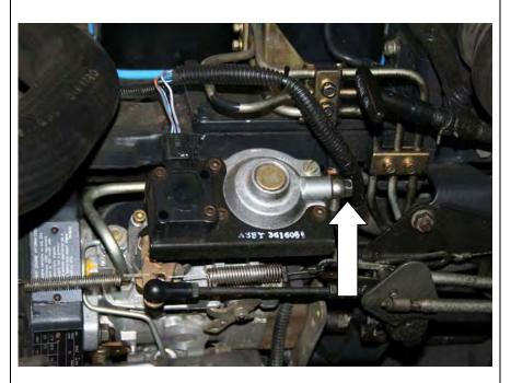
3. Remove APPS Sensor and bracket. Manual transmissions do not have an APPS.
