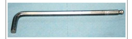
9. Using the rounded end of the allen key remove the 4 bolts holding the cover on. You will need to use a wrench on the end of the allen key as the bolts are quite tight.
