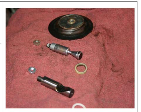
9. Before inserting new pin assembly, stroke the throttle linkage back and forth <u>slightly</u>. You can use some lubrication at the same time to assist you.
