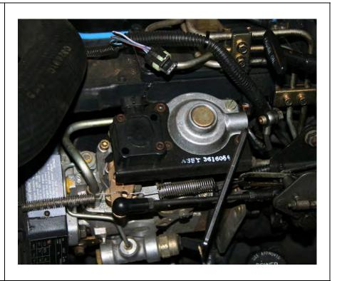
14. Re-install the 12mm Banjo bolt at the rear of the AFC.
