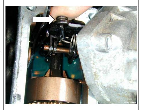
15. Install the throttle shaft spring assembly. Hook the bottom spring hook in and then the lower plastic piece will hold it in place. Pull up on the throttle shaft to get it in position.
