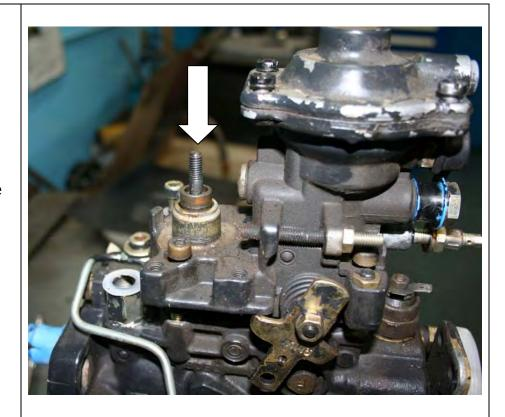
11. With the cover off you can now access the governor spring. Using your fingers just replace the spring. Be careful as one end is under spring tension.
