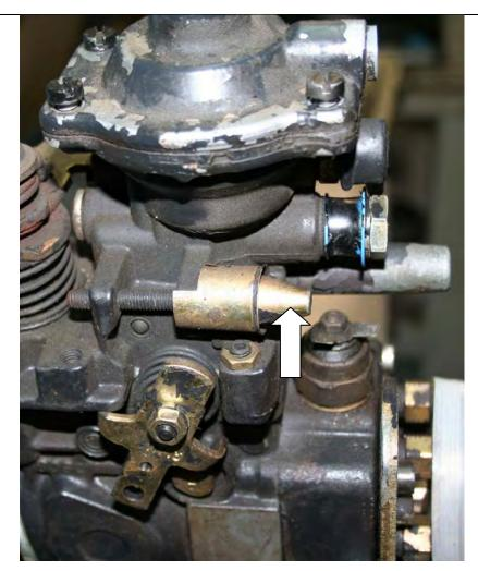
5. Using a 10mm socket, remove the jam nut that secures the reminder of the tamper proof cap. Throw away tamper proof cap pieces.
