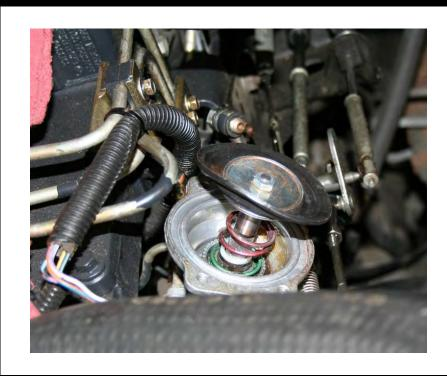
11. Ensure the ground fuel pin profile faces directly forward. To ensure this, lift the fuel pin assembly slightly and stroke the accelerator linkage from 0% to 100%. Do this while twisting the fuel pin slightly. You will feel a point of no resistance or when the rotational movement comes to a center point. This is the correct alignment.
