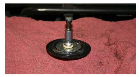
7. Remove the factory fuel pin from the diaphragm by using two 10mm wrenches. One on the jam nut the other on the rectangular slots on the fuel pin.
