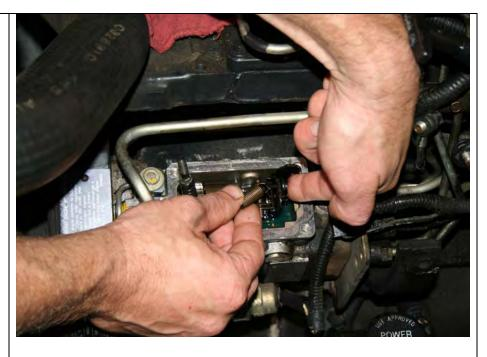
12. Replace oring on throttle shaft, with the oring supplied (#1505020).
