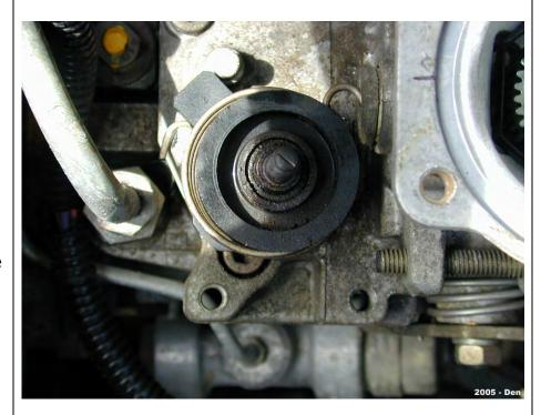
4. Remove the tamper proof cap on the high idle screw. Simply grab the cap with pliers or vice grips and pull towards the rear of the vehicle.
