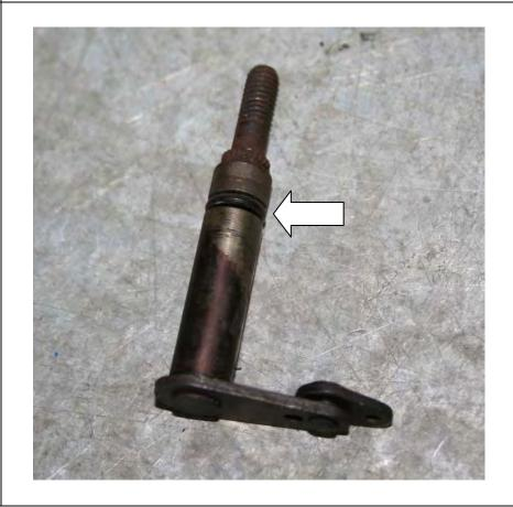
13. Slide the throttle shaft through the top cover.
