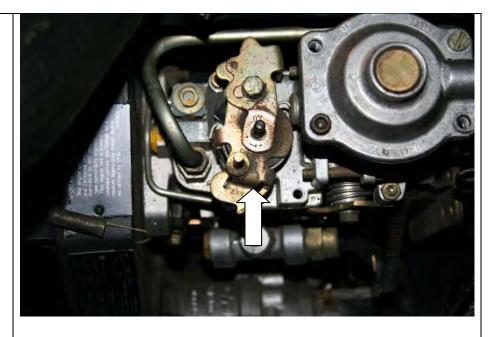
3. Remove the throttle return spring as well as the 2 plastic parts (top and bottom). Lift these off in one piece as they have to go back in place in the same order.
