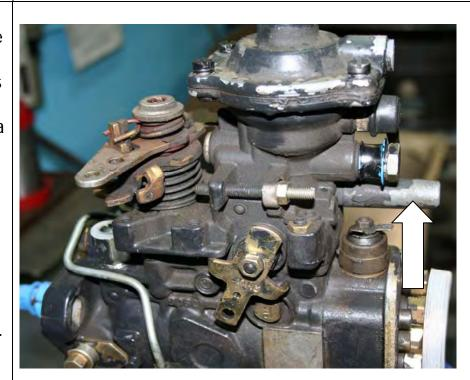
7. With the tamper proof cap removed, back the screw out until the oring is visible.
