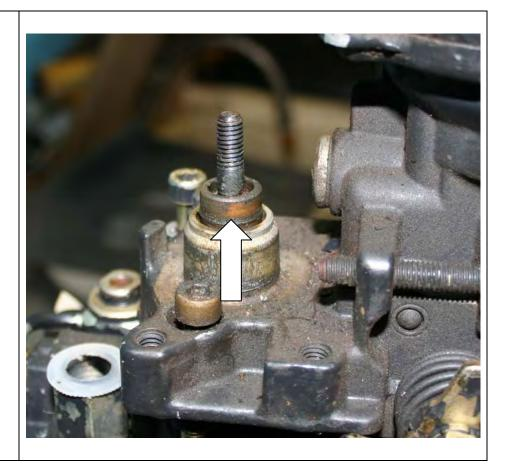
14. With the spring back in place, hold the governor spring assembly in position so that you can replace the top cover. Tighten the four cap screw bolts.
