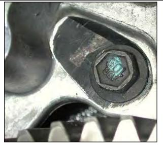
With retainer and bolt installed
