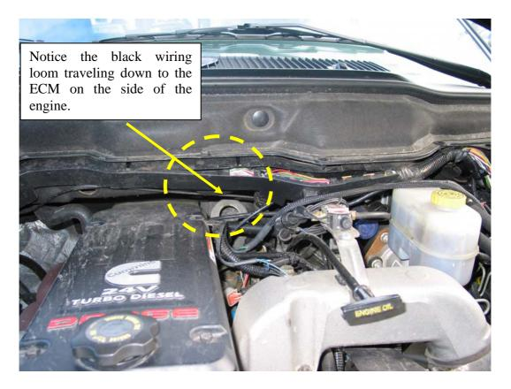
3. There will be a white w/orange tracer wire as well as a violet w/yellow tracer traveling down to the ECM inside this wiring harness. These are the wires you must cut, be sure to leave yourself enough room to crimp on connectors when cutting these wires.
