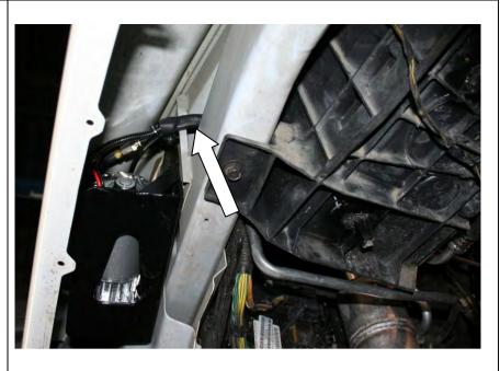
Use the wiring diagram on page 19 as a reference for the wiring of the air hoses and the electrical wiring. NOTE: Be sure to keep all hoses and wiring harnesses away from any moving parts or heat sources.
