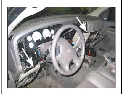
Drill a pilot hole with a 1/8" bit and finish by enlarging the hole with a Unibit to exactly 1/2".
