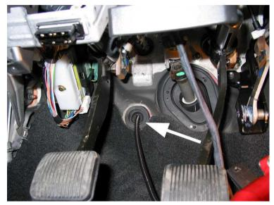
Open the loom and locate the Light Blue w/Black wire and install a supplied Posi-Tap™ to it.
