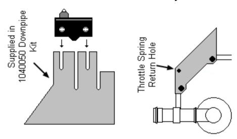
Connect a length of the supplied wire from the "com" terminal on the micro switch to the red wire on the spool valve. Run another length of wire from the "NO" (Normally Open) terminal through the firewall. This will be connected later.
