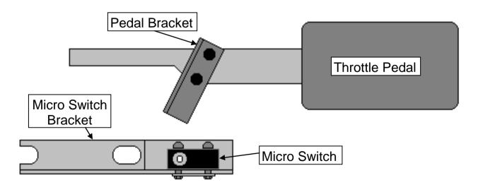
Connect a length of the supplied wire from the "com" terminal on the micro switch to the red wire on the spool valve. Run another length of wire from the "NO" (Normally Open) terminal through the firewall. This will be connected later.
