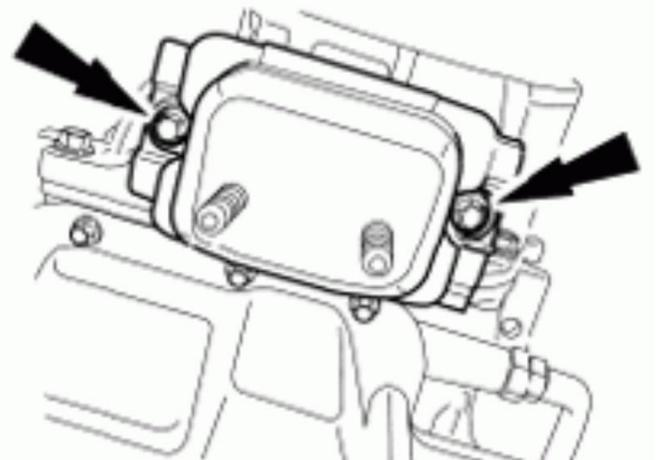
9. Loosen the bolt and disconnect the transmission vehicle harness connector.
