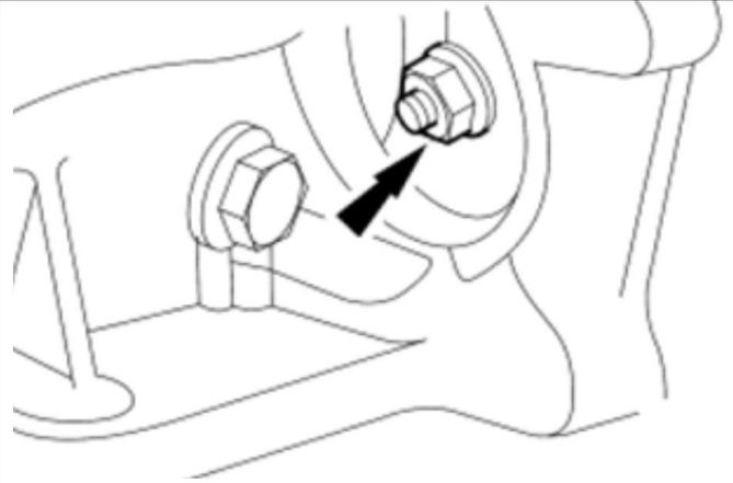
20. Remove the 9 transmission-to-engine mounting bolts.
