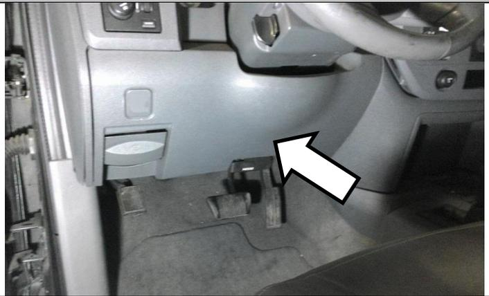
Remove the steering wheel tilt lever using a T20 screwdriver.
