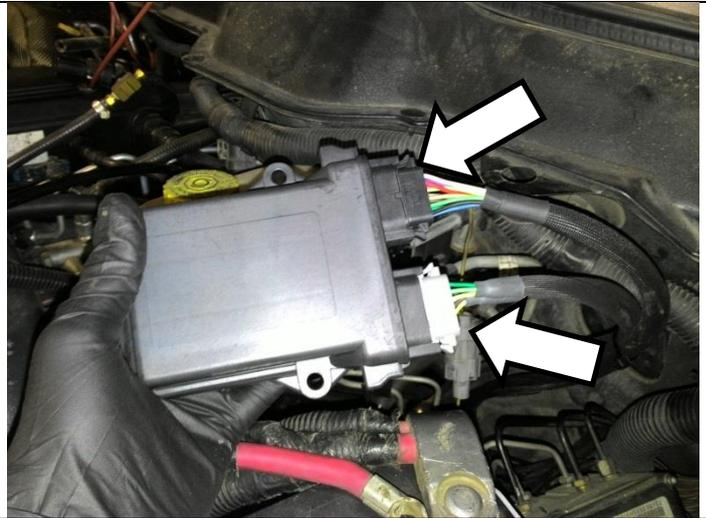
Mount the module using wire ties in the engine bay. Here we show it attached to the engine wiring harness on the driver's side of the firewall.
