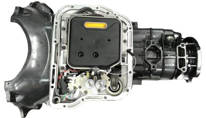
**Important** Check to ensure the steel tube support bracket is still in place and adequately supporting the tube. It may have been moved the previous steps.
