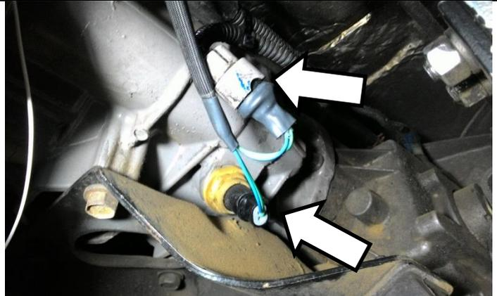
Locate the 8 pin electrical solenoid connector for the transmission, ahead of the speed sensor. Unplug the connector.
