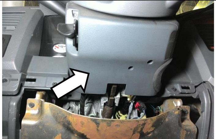
Using a trim removal tool, pop off the transmission shift cable from the shift lever.
