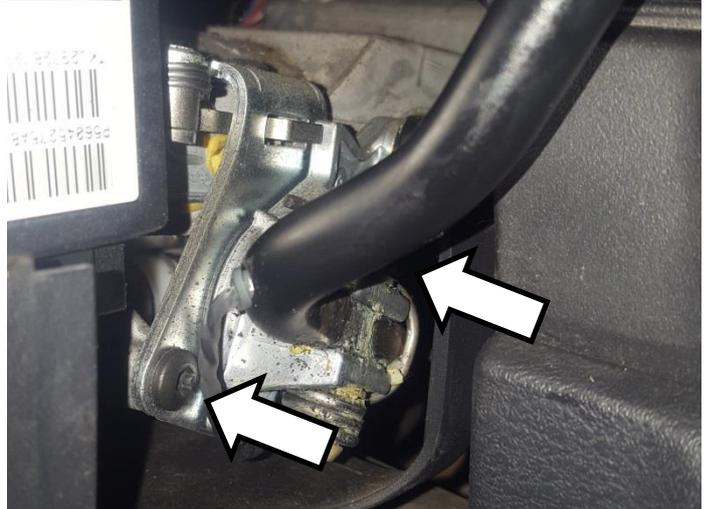
The remaining fastener is located on the top of the column. If you do not have a small T27 bit and ratchet, removal of the instrument cluster surround may be necessary to remove this screw.
