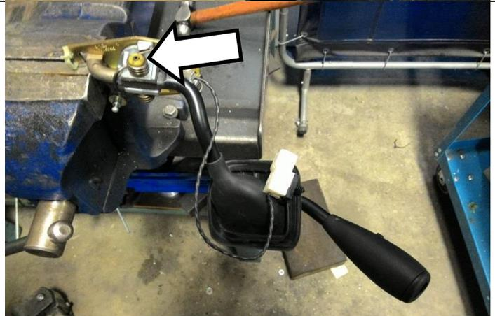
Reinstall the shift lever in the truck. Rotate the lever into place so that the shifter lock mechanism is in place. Install the three Torx fasteners removed earlier.
