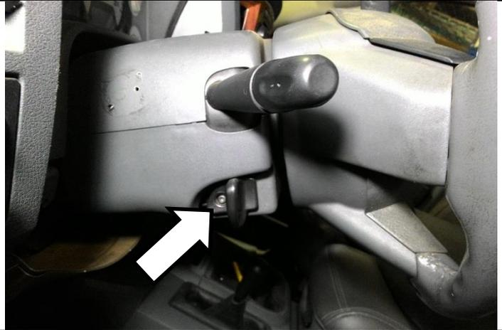
Remove the screws from the bottom of the steering column covers and remove the plastic covers.
