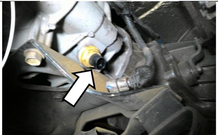
Connect the BD harness to the speed sensor and plug the stock wiring into the BD harness.
