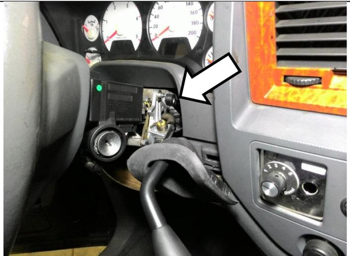
Route the thin twisted wire from the shift handle in the same routing as the original shift lever. Put the wire in the original support clip and push in the Christmas tree clip. Ensure the wire does not impede shift lever movement and that the wire will not become chaffed.
