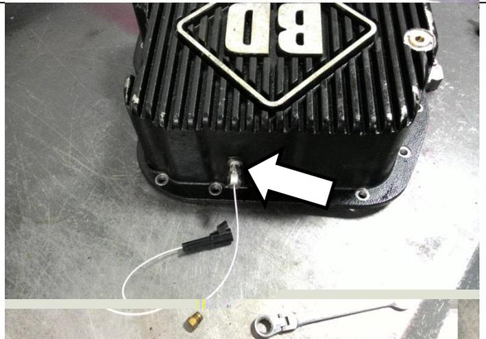
Raise the transmission pan below the transmission and connect the one pin connector from the governor solenoid wiring to the through pan wiring harness.
