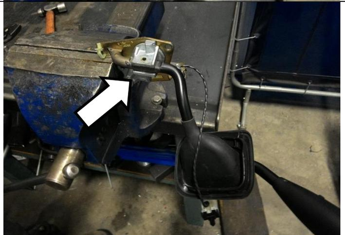
Reposition the spring and bushings for installation.
