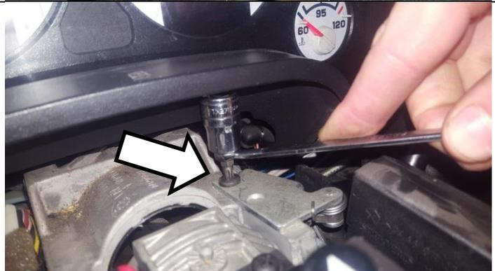
Remove the shift lever assembly from the column. The shifter assembly needs to be rotated to release it from the shifter locking mechanism.
