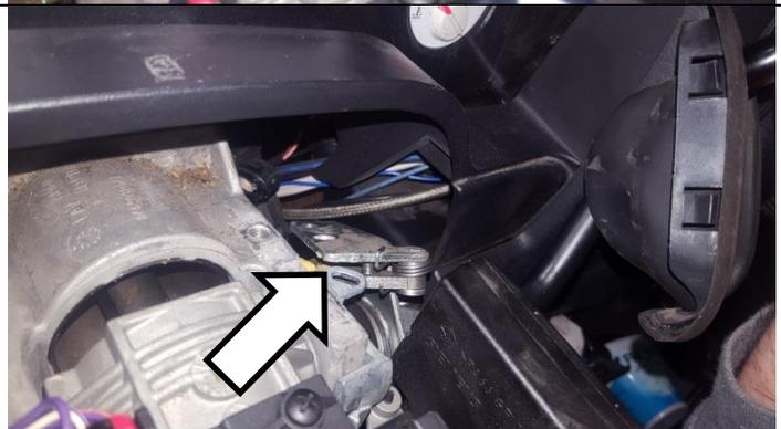
Take the shift lever over to a work bench with a vice. The next steps will involve transferring the new handle (5057438AC-P) into the original bracket.
