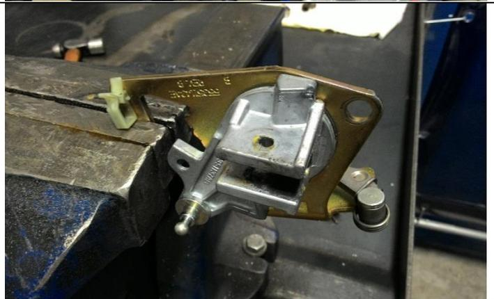
Apply a small amount of grease to the new shift lever in the area that it will contact the shifter bracket and slide it into the bracket in the same orientation as the old lever.
