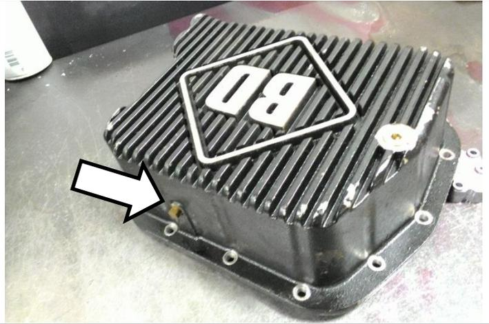
Feed the small end of the wire harness from the outside of the transmission pan to the inside.
