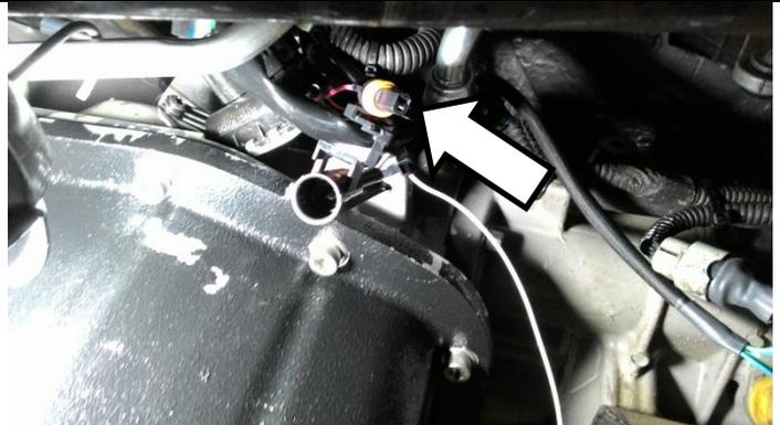
The BD transmission harness should be supported along the same route as the factory wiring harness and should be attached with wire ties to ensure it does not get near any moving parts and does not put significant strain on any of the wiring connectors.
