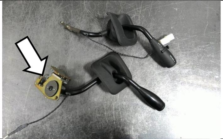
Mount the old shifter bracket in a vice and use a punch or other suitable tool to drive the shifter pin out.
