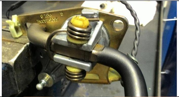
To start the pin you must squeeze the spring, moving the bushing into alignment.
