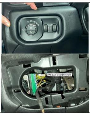
The white connector can be plugged into any open port of the StarCAN C junction (green connectors with black housing) as shown.
