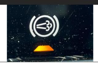
The exhaust brake functions just like the factory exhaust brake. Pressing the exhaust brake button cycles between full and automatic modes.
