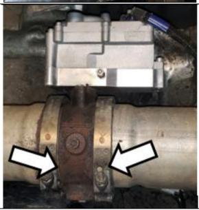
Weld the front adapter to the exhaust pipe. This weld must completely seal the exhaust system as it must retain pressure.
