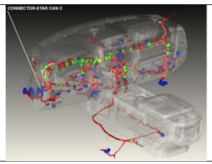
2018: This can be located by looking up from the pedals towards the instrument cluster.
