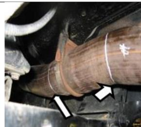
Cut out the marked pipe section using a reciprocating saw or cutting disk. Remove any burrs left on the edge of the pipe using a file or similar tool, then slide the pipe adapters onto the two cut ends of the pipe.
