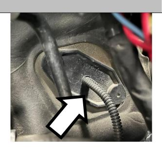
Locate the StarCAN connector on the driver's side of the dashboard behind the headlight controls.
