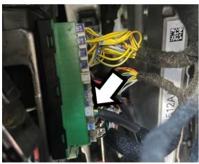
2019: This can be located by looking up from the pedals towards the instrument cluster. Alternatively, use a pry tool to release the headlight control cluster to reveal the StarCAN connector as shown.
