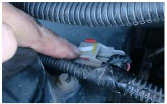
22. Disconnect the EGR servo motor connector.
