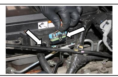
13. Using a puller tool pull out the harness clips that secure the harness to the grid heater and the other clip on the backside of the valve cover.
