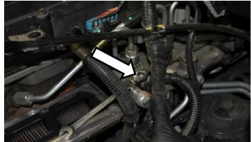
7. Install the heater cable to grid heater stud using the supplied Nyloc nut. Tighten to 9 ft-lbs (12.2 Nm).
