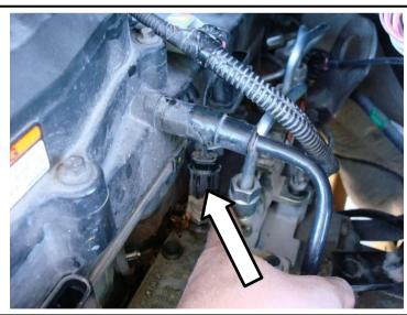
21. Disconnect CCV pressure sensor harness connector that is located at rear of the valve cover. This needs to be disconnected to allow you to coil the harness aside to access the grid heater.
