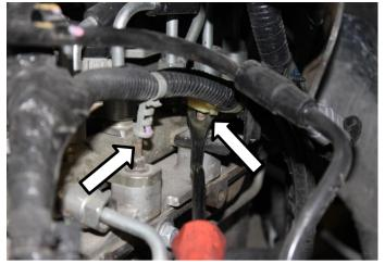
12. Reconnect the throttle valve sensor to the bottom of the intake horn.
