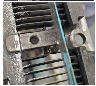
6. Install the nylon insulating washer to the bottom of the grid plate with the washer shoulder inserted into the bolt hole.
