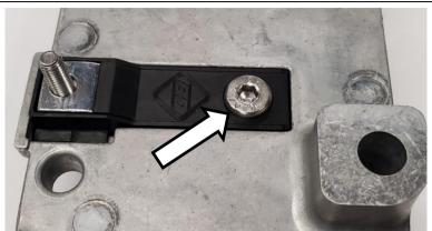
11. Tighten the lower busbar bolt to the heating elements to 7 ft-lbs (9.5 Nm).
