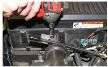
16. For 2013+ models: Reinstall the heatshield covering the intake control valve.
