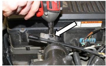
5. For 2013+ models: Remove the heatshield covering the intake control valve.
