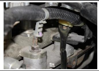
14. For 2013+ Models: Remove the sound deadening foam rubber from around the fuel injection lines to allow access to the fuel lines.
