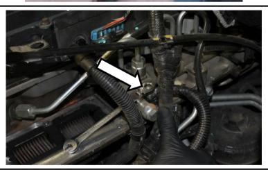
24. Remove the four bolts holding the fuel rail to the grid heater (10mm).
