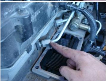
20. Disconnect the intake air temperature sensor connector from the grid heater.
