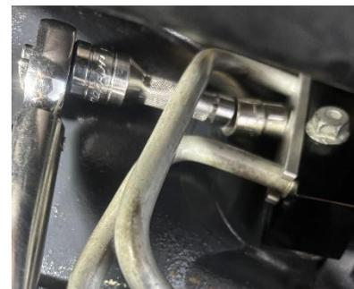
Correct transmission fluid level and check for leaks.
