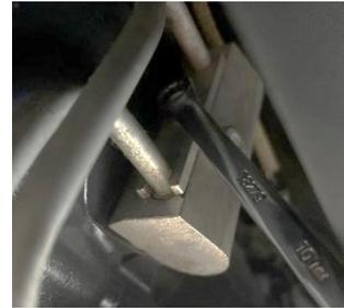
Pull out the cooler lines from the thermostat block.
