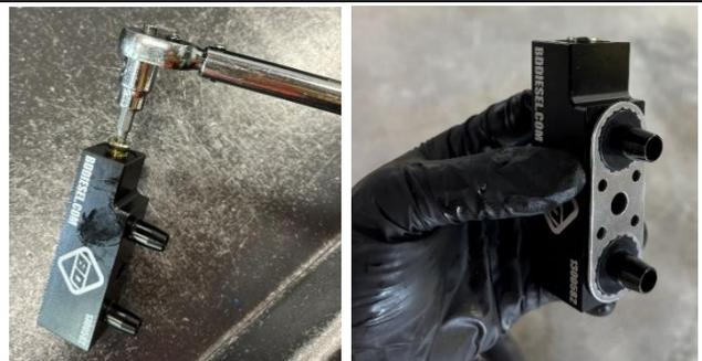
Clean the block gasket surface on the transmission, and install the bypass block with the plug upward.
