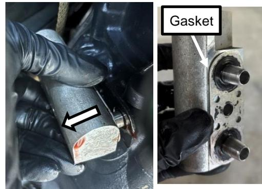
Using a **3/16"** Hex bit, install the magnetic drain plug (1453160) into the bypass block.
