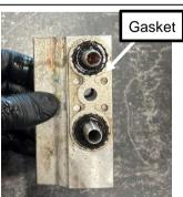
Using a **3/16**" Hex bit, install the magnetic drain plug (1453170) into the bypass block.
