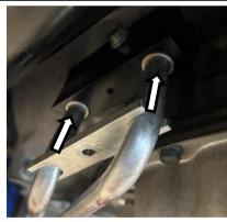
Using a **10mm** socket, install the transmission fluid cooler pipe retaining bolt through the retaining plate and into the bypass block.
