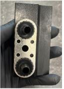
Clean the block gasket surface on the transmission, and install the bypass block with the cooler line ports facing downward.
