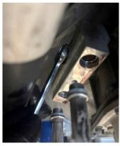
Remove the thermostat block and gasket from the transmission.
