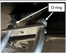
Insert the cooler lines into the bypass block.
