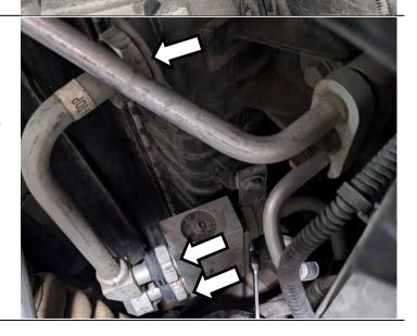
Using a 10mm wrench, remove the fastener holding the retainer plate to the bypass block.
