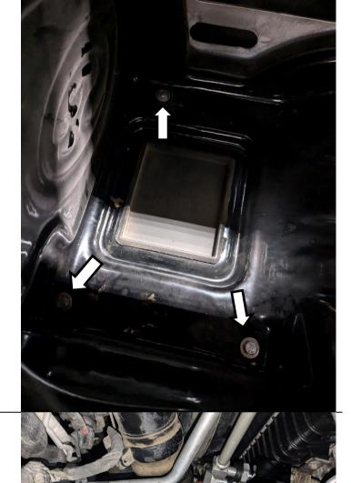
Remove the 5x lower air box support bracket fasteners using a 10mm socket.
