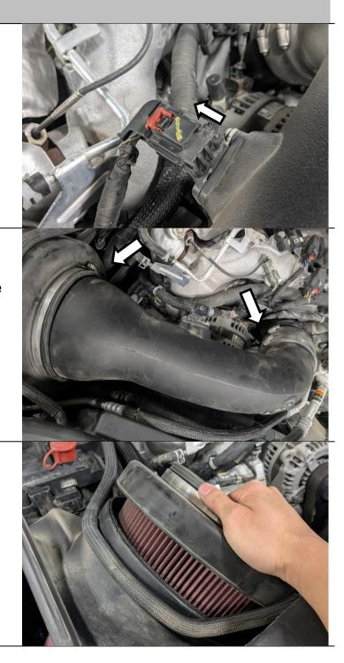
Remove the 3x air box fasteners using a 10mm socket.
