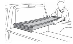
**NOTE**: IF TONNEAU IS SITTING TO HIGH ON TRUCK BED RAILS, REMOVE FOAM TAPE ON FRONT RAIL UNTIL DESIRED HEIGHT IS ACHEIVED.
