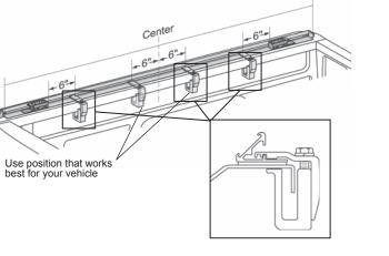
in so they are flush with the Front Rail. Center the front of the Frame from side
