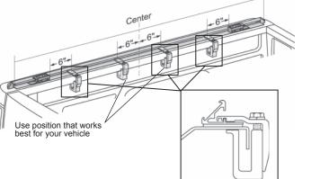
With the Tonneau Cover Assembly latched on both sides, push both Side Rails in so they are flush with the Front Rail. Center the front of the Frame from side to side on the vehicle.
