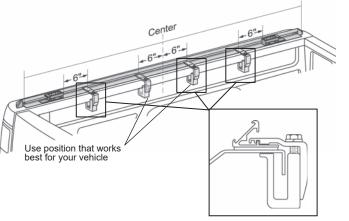
in so they are flush with the Front Rail. Center the front of the Frame from side
