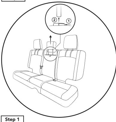
Remove the center console headrest. Lift the headrest until it stops. Then:
