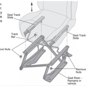
**WARNING** DO NOT reuse the original mounting bolts. Reuse of the bolts could cause the seat to loosen, which could result in loss of control of the vehicle, causing bodily injury to the vehicle occupants and to others.
