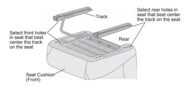
**WARNING** Use only the bolts provided in the Parts Kit when installing the new seat. Failure to do so may cause the seat to loosen, resulting in loss of control of the vehicle and causing serious bodily injury to the vehicle occupants and to others.
