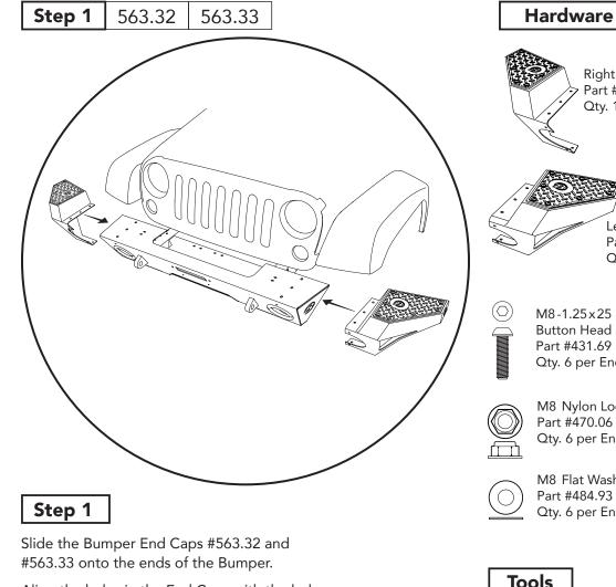
Align the holes in the End Caps with the holes in the Bumper.
