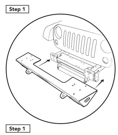
Re-Attach the Front Bumper. The studs on the inside of the Bumper will fit through the holes in the bumper mounting plates and through the holes in the Inner Roller Brackets.
