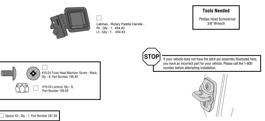
**Special Note:** The Rotary Latch Paddle Handle **will only** latch on the automobile manufacturer's original equipment steel latch pin located on the vehicle. **Do Not adjust or remove this part.**
